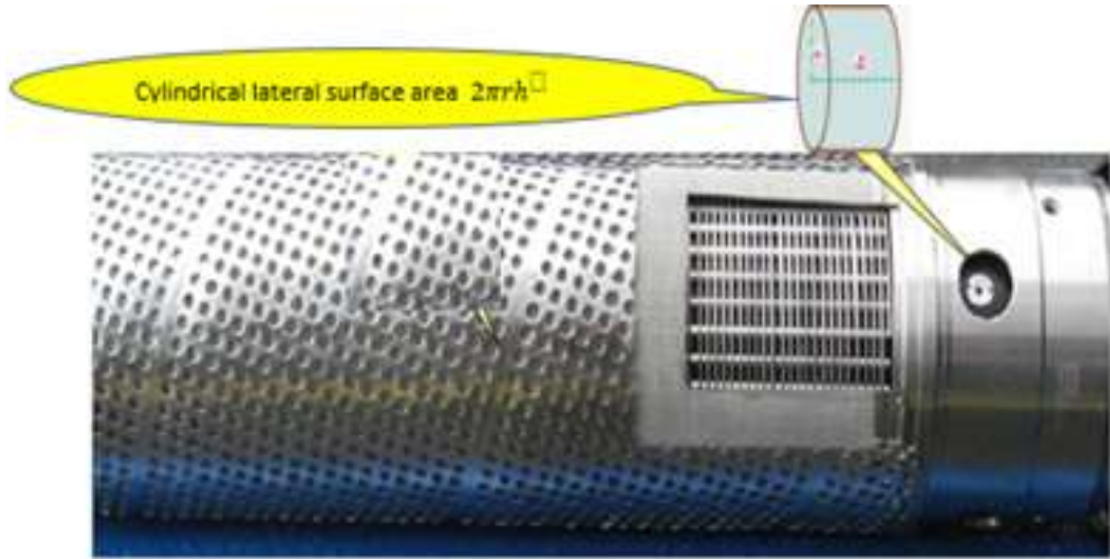
Figure 6. showing lateral surface area of each cylindrical shape ICD nozzle in each segment of a horizontal well.
